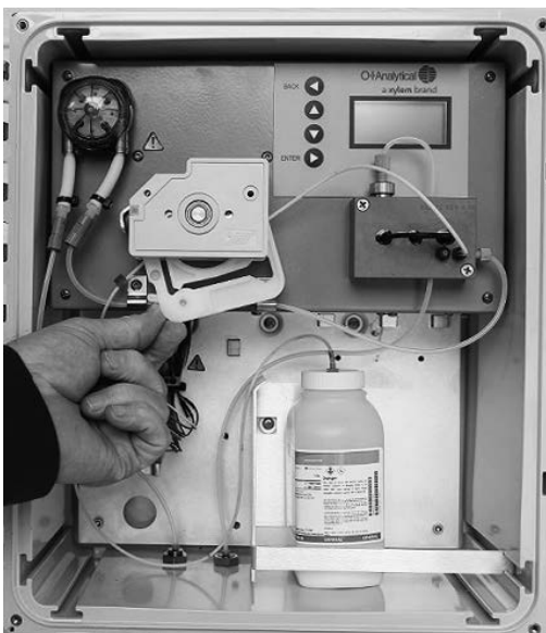
Figure 6.3 Installation of buffer reagent tube
