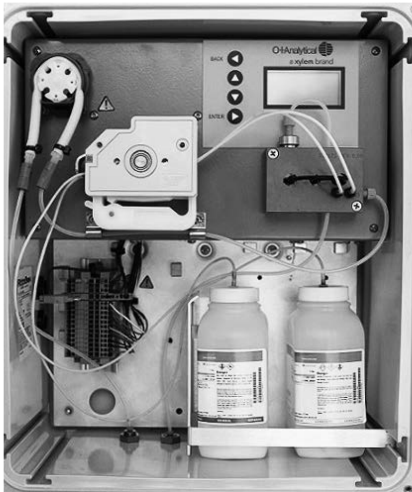
Figure 2.9 Installation of the sample pump tube
