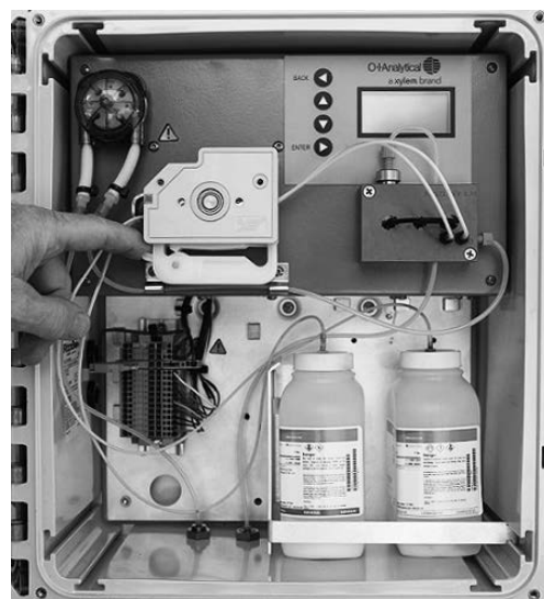
Figure 6.4 Completed reagent tube installation and platen tensioning
